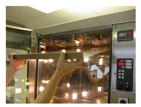
... And slide the cover out from the oven cavity.
